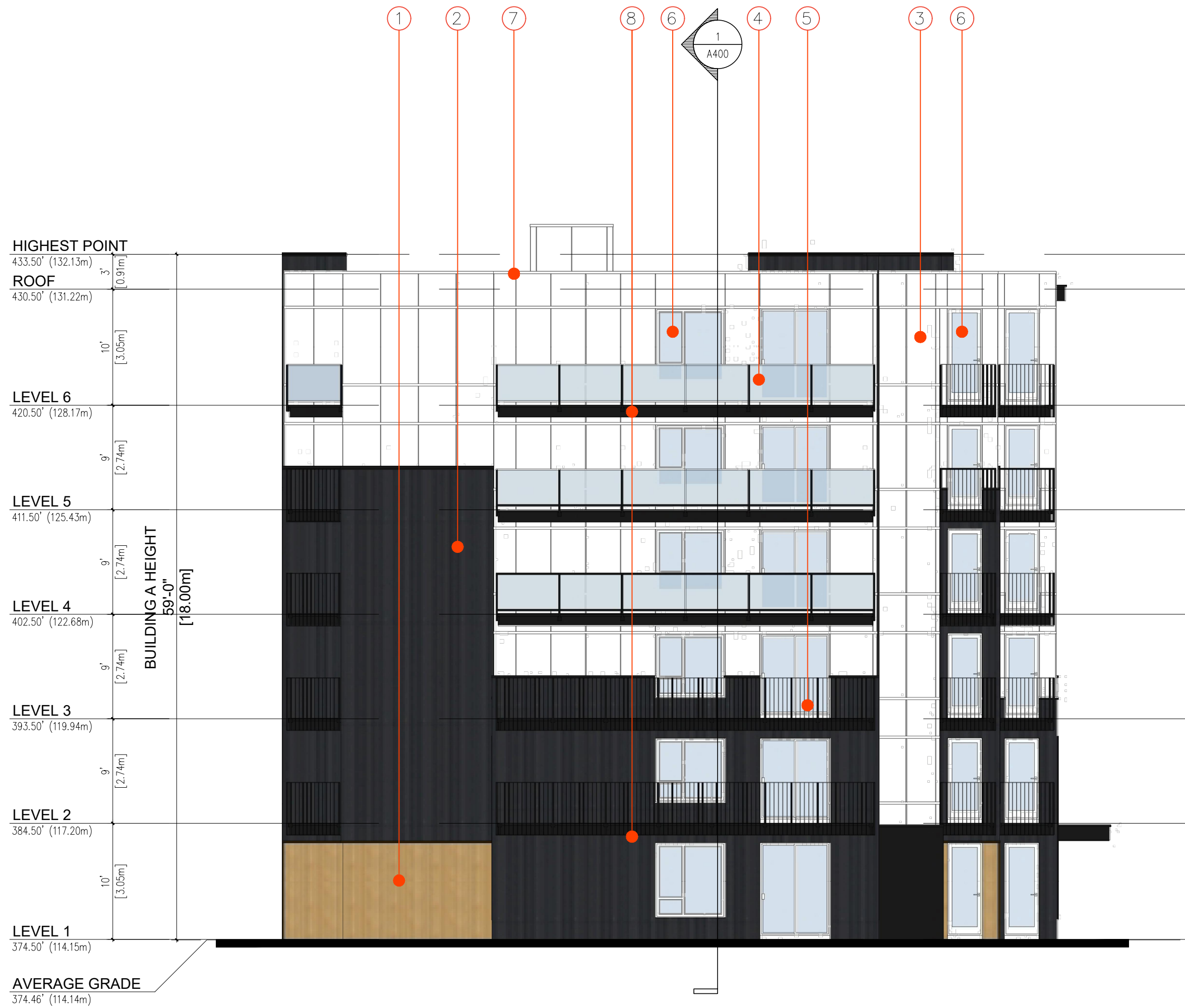
2 BUILDING A - SOUTH ELEVATION 1:100
